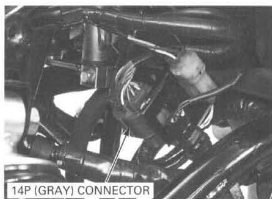
COMBINATION METER 14P (GRAY) CONNECTOR (Wire side of male terminal)
